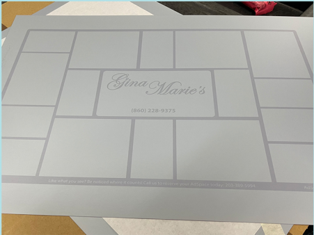
A printing plate for a placemat
